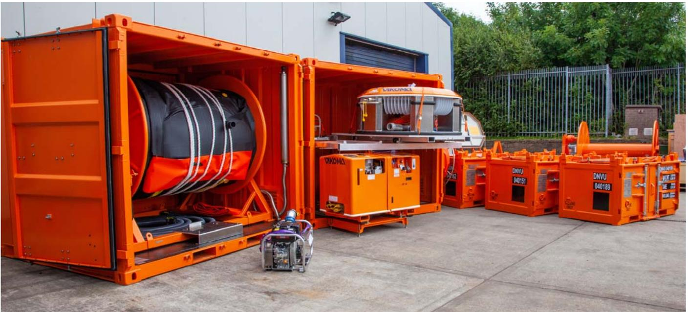
*Containerised package for FPSO comprising Neoprene Hi Sprint Oil containment boom, Komara Maxi oil skimmer, Powerpack and inflatable oil storage barges in offshore containers.*
