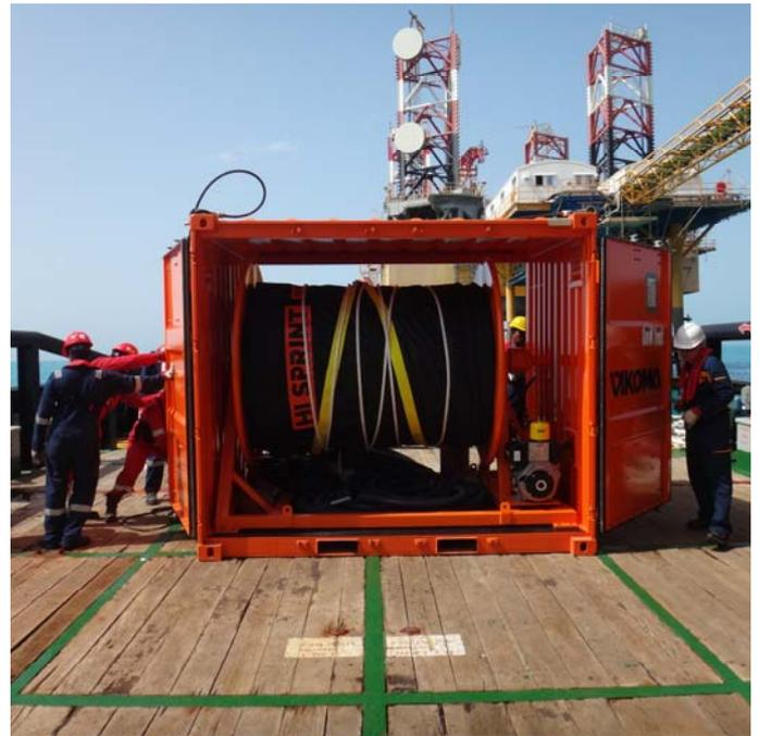
*Containerised neoprene Hi Sprint oil containment boom system on a boat*
