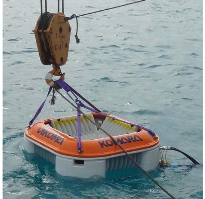
*Komara Midi 4 being deployed by a crane from a boat*
