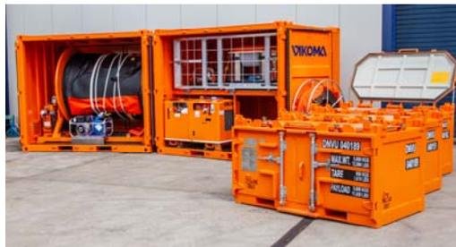
*Containerised package of oil spill equipment for offshore use*
