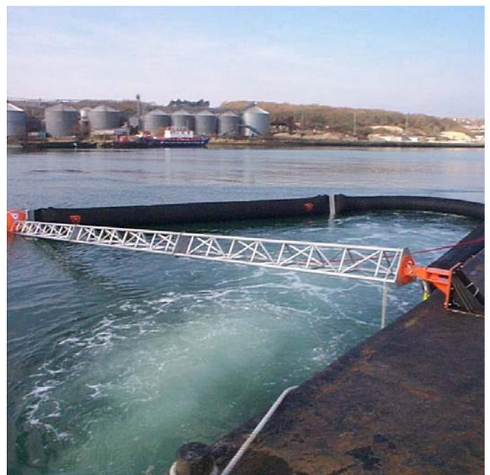
*Sweep arm attached to a neoprene containment boom*
