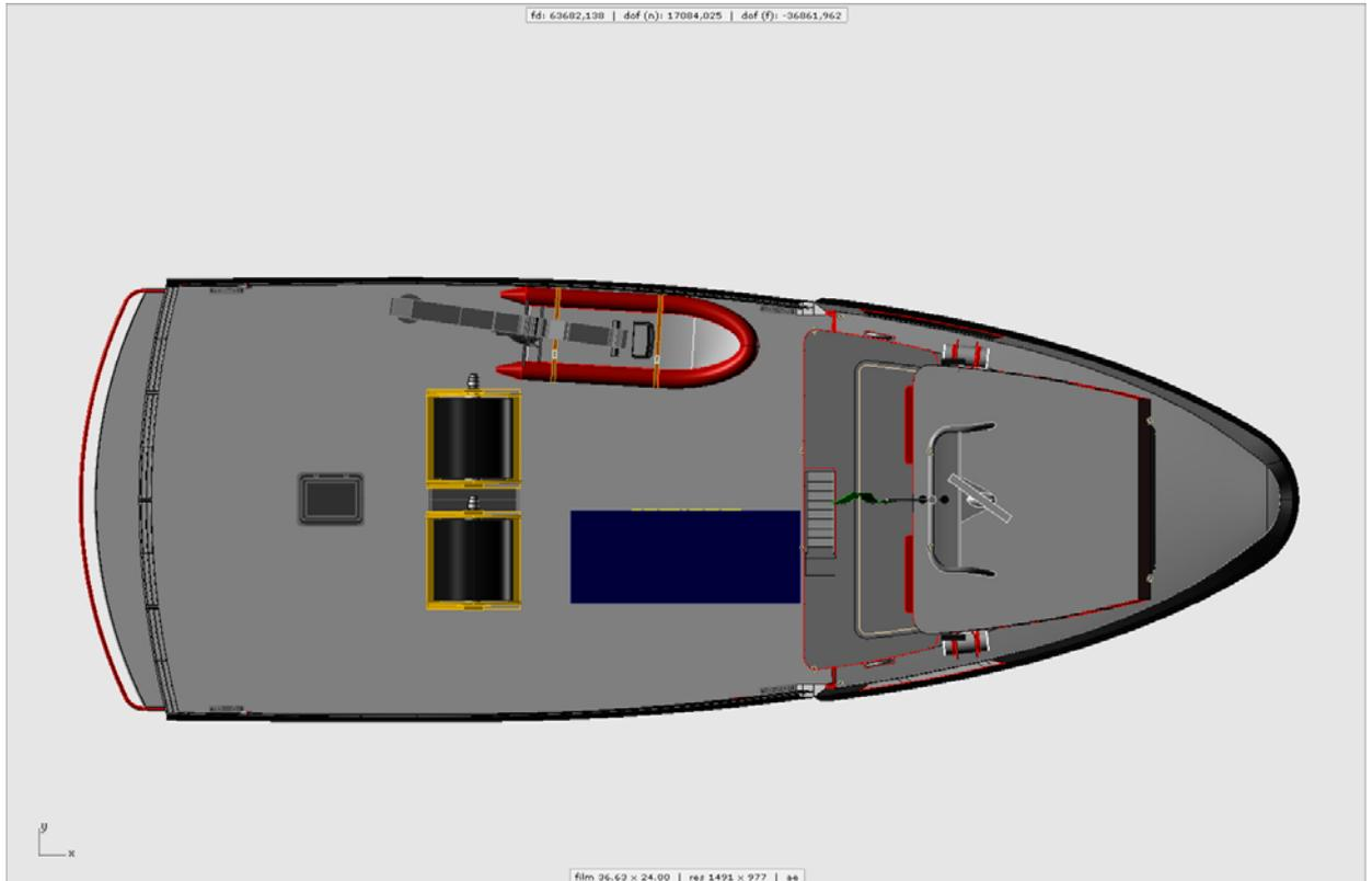
The basic model of the vessel is not constructed for navigation in ice field. However, we have tested the trimaran hull in arctic laboratory and know that when the hull is properly strengthened, the 30 m version can go in 25cm ice. The shape has been patented for navigation in ice conditions. The navigation ability in Nordic waters will be offered as an option
